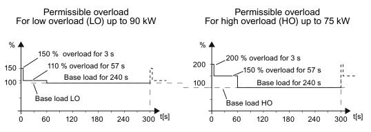
Figure 6-1 Duty cycles, "High Overload" and "Low Overload"
