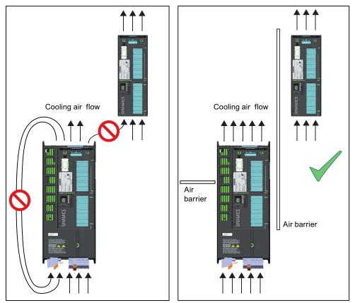
5. Avoid short circuits of the cooling air using air barriers, if necessary
