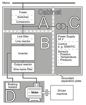
Zone A: Supply connection Limit values for conducted interference emissions and conducted interference immunity must not be exceeded
