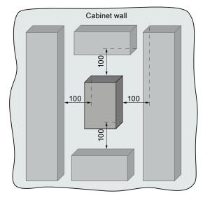
Figure 7-2 Distances to other equipment [mm]
