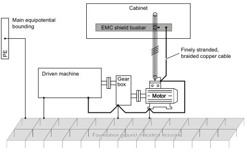
Figure 4-2 Additional high-frequency bonding of the drive system
