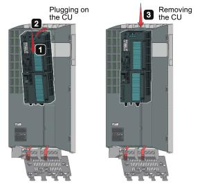
Fitting the Control Unit to the Power Module
