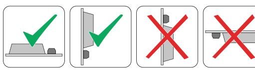
Figure 7-3 Permissible mounting orientation of the braking resistor
