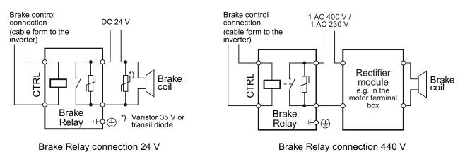
The Brake Relay has to be connected to protective earth, if the motor brake is supplied by a PELV circuit.
