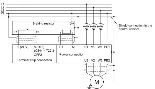
Figure 7-5 Braking resistor connections (Example: temperature monitoring via DI 3)
