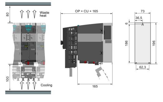
For fixing: Screws M4, 2.5 Nm
