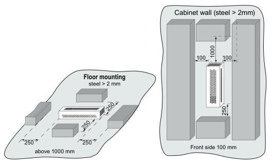
Mount the resistor on a heat resistant surface with a high thermal conductivity. Do not install devices that could impede the flow of cooling air in this area. Do not cover the ventilation openings of the braking resistor.
