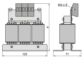
a = 120 mm for Low output Power 0.55 kW ... 1.5 kW a = 140 mm for Low output Power 2.2 kW ... 3.0 kW
