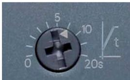
You define the length of the required ramp time with the t potentiometer. The ramp time determines the time taken to increase the motor voltage from the parameterized starting voltage to the mains voltage. This time merely influences the motor's acceleration torque, which drives the load during the ramp-up process. The actual motor starting times are load-dependent and can differ from the 3RW soft starter settings.
