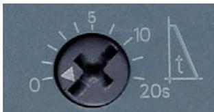
You can set a ramp-down time with the t potentiometer. This determines how long power should still be supplied to the motor after the ON command is removed. The torque generated in the motor is reduced by means of a voltage ramp function within this ramp-down time and the application stops smoothly.
