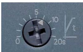
You define the length of the required ramp time with the t potentiometer. The ramp time determines the time taken to increase the motor voltage from the parameterized starting voltage to the mains voltage. This time merely influences the motor's acceleration torque, which drives the load during the ramp-up process. The actual motor starting times are load-dependent and can differ from the 3RW soft starter settings.
