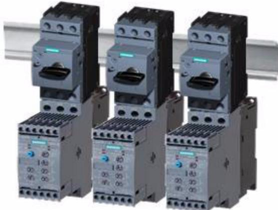
The term "direct mounting" is used if the top clearance  $b$  described in chapter Mounting dimensions, clearances, and assembly type [Page 54] is not complied with, e.g. if the soft starter is mounted directly on a motor starter protector (e.g. 3RV2) using a link module (e.g. 3RV29).
