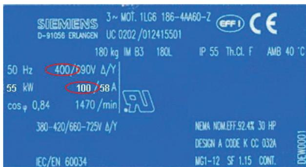
The rated operational current of the motor must be set with the  $I_e$  potentiometer according to the mains voltage and the motor connection (wye-delta). The electronic motor overload
