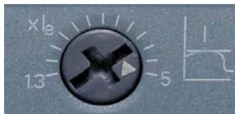
The current limiting value is set with the  $xI_e$  potentiometer to the maximum required starting current as a factor of the set rated motor current ( $I_e$ ).
