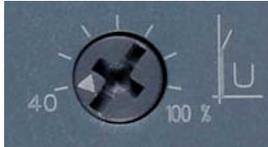
The starting voltage value is set with the U potentiometer. This value determines the starting torque of the motor. A lower starting voltage results in a lower starting torque (softer start) and a lower starting current.
