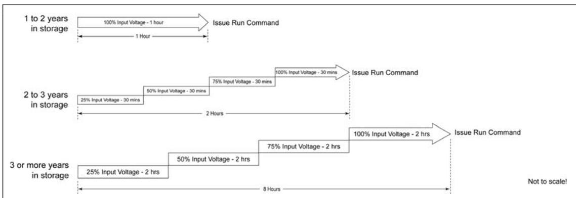
Figure 2-1 Reforming Capacitors After a Period of Storage
