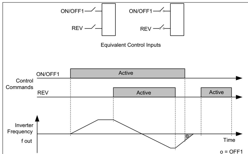
Figure 4-1 Siemens standard control using ON/OFF1 and REV
