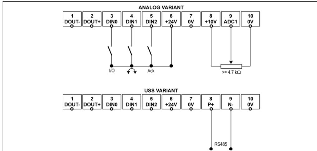
Figure 3-3 Basic operation – Analog and USS Variants
