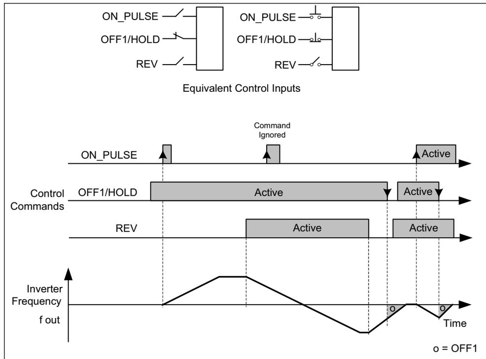
Figure 4-5 3-wire control using ON\_PULSE, OFF1/HOLD and REV
