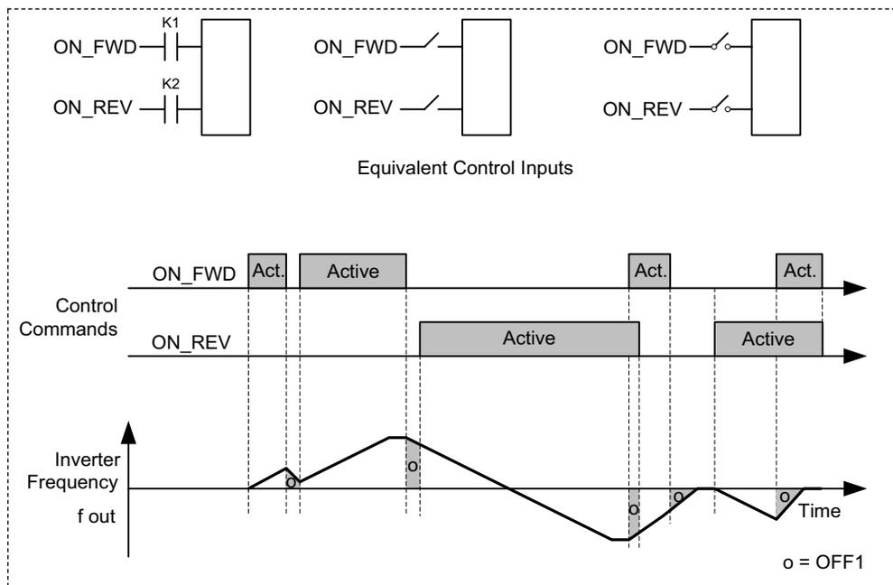
Figure 4-3 2-wire control using ON\_FWD and ON\_REV
