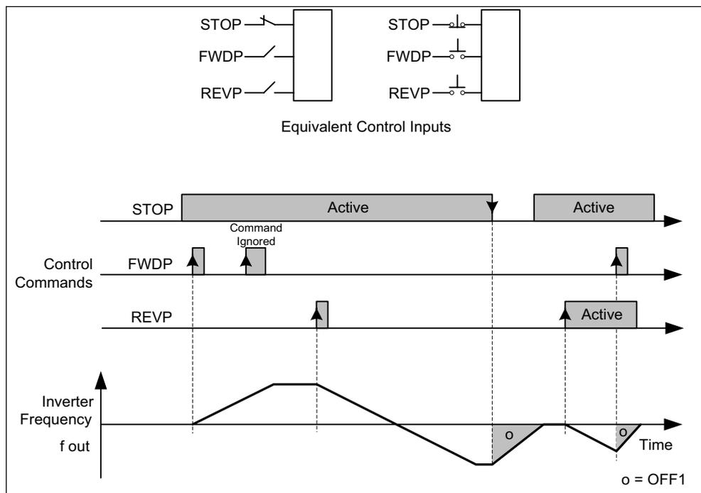
Figure 4-4 3-wire control using FWDP, REVP and STOP
