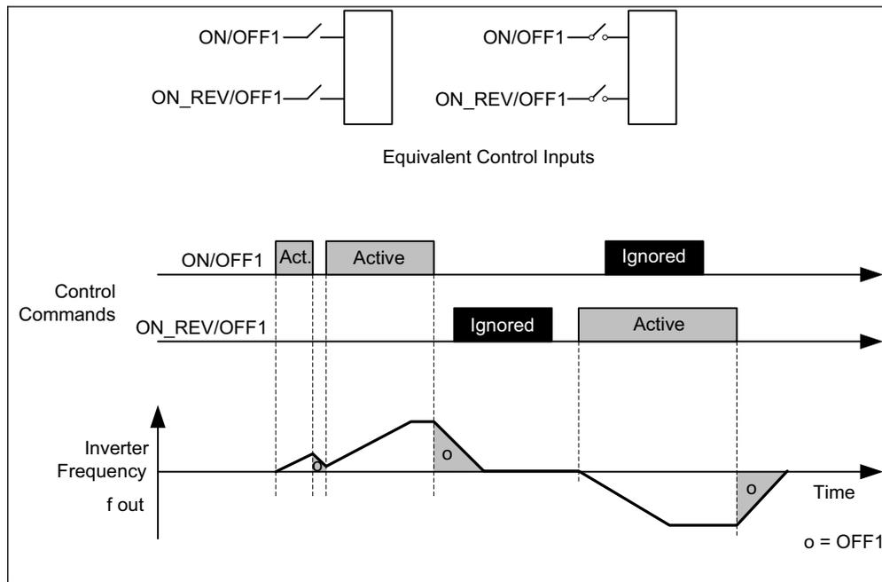
Figure 4-2 Siemens standard control using ON/OFF1 and ON\_REV/OFF1
