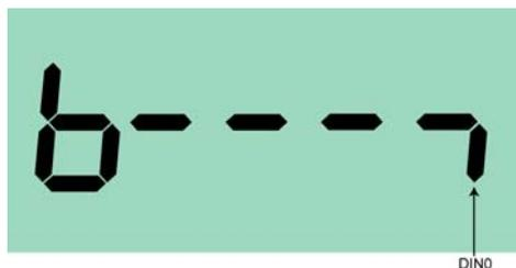
5. The lower mark on the right-hand side of the display indicates that DIN0 is active high, that is, an ON command is present.
